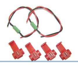
When switching from 5 Watt indicator, position or rear light bulbs to LED bulbs, the power consumption will be lower than normal. You might experience error messages on some newer cars with canbus or bulb-control. Because of this you will need to apply these "cheat resistors", which raises the consumption, so that it matches a regular bulb.
