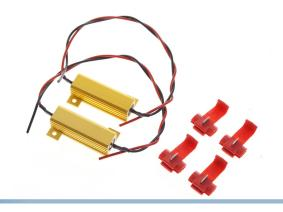
When switching the fog/tail lights with LED styling lamps or the diode bulbs, the power consumption will be lower than usual and thare can be therefore experienced error messages on some newer cars with Can-Bus or bulb-control. You will therefore need to apply these "cheat resistors", which raise the consumption, so that it matches a regular bulb. The resistors will be connected to the + and - approach from the car.
