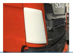
Dirt deflectors for Scania Next Genration S / R-series with a custom-made design. All the mounting screws are hidden on the backside of the deflector and is very easy to mount.
