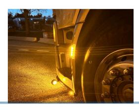
Simple adapter, so that you can use the indicators on the side of the cabin, as a position light. The brightness will be dimmed compared to the indicator light. The indicator will work as usual with its high brightness, and it is still highly visible due to the difference in brightness.
