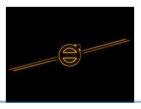
Lightbase for the diagonal lines, on the sides of the Volvo-logo. The original lines fits in to the base, where they are glued in place.
