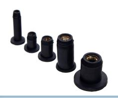
Nut in rubber housing, for fastening parts on a surface, where you cannot get access to use a normal nut on the backside. The Ø-dimension on the variants are the hole-diameter they fit in to.
