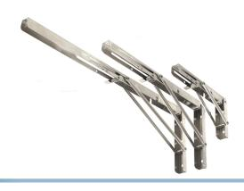
Compact bracket that is unfolded and locks itself at 90 degrees, A push on the handle and it can be folded back again. While they are in our System profile category, they can be used for any purpose, eg. mounting directly to a wall, with a shelf board on top.
