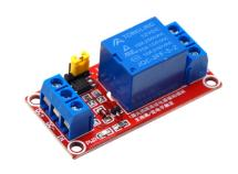
Simple relay module that can be used where you have a low-voltage-signal, that has to turn on or off a higher voltage.
