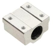
Linear block for 8mm axle, with holes for mounting of part, typically called SC8UU. There are 4 rows of balls inside the block, which gives you an even and precise movement.
