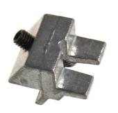
Simple holder for fence and net, that fits in to series 30 and 40 profiles. When the net is in place in the track, you simply place this around a wire. When you tighten the pinol screw, it locks itself and the net in the track.
