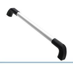
Large handle for series 40 profiles. The anodized Ø30mm aluminum tube can be cut off to the wanted length and is then put into the ends, which are fastened with M8 bolts. The plastic ends are made of reinforced nylon for maximum durability.
