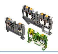
Clever feed-through terminal blocks for mounting on DIN rail. The terminal blocks have push-in terminals, that make it easy to connect. The terminals can be used for  $0.14~\text{mm}^2$  -  $4~\text{mm}^2$  wires.
