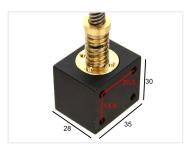
Housing in aluminium for M8 trapez nuts. Nut is mounted with 2 x M3 screws, housing is mounted with  $4 \times M4$  threaded holes in the bottom.
