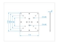
Standard Vesa monitor bracket in solid anodized aluminum. Can be mounted directly on profiles, on bracket and arms. You need M4 bolts for mounting the plate on the screen, and possibly also spacers, washers or nuts.
