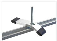
Standard profile in our T-track system, that fits the sliders and t-nuts from the same system. The profile-dimensions are  $30 \times 12.8 \text{mm}$  with 19.3mm track width.
