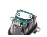
Caps in aluminium, that you can be "turn off" the LED emitter in the DRL on Scania +2016, can be used if you want to use other DRL lamps.
