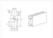
Strong profile that is intended for lids, doors and other parts that demand high stiffness. The profiles has tracks on the slim sides, and completely blank on the others.
