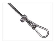
Thimble that is used for protecting a wire-loop against wear. It is inserted into the joint, and prevents the part put through the loop from wearing the strands.
