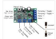
Smart protection against high current, that can be used for protecting motors, actuators and other similar current-variable units. When you block a motor or an actuator, it will use an extra high current, which very quickly can result in the motor overheating and be destroyed. This protection can prevent this, by shutting the power off.
