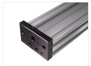
Plate that can be bolted on to the end of a C-beam profile, where it can be used for mounting a NEMA 23 motor and a lead screw to the profile.
