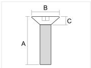
Countersunk bolt for mounting in countersunk holes. Used when you want a flat mounting surface.
