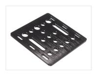
Gantry plate for v-slot tracks, that are 20mm wide, eg. 2020. og 2040. Used together with standard v-slot wheels. The plate is made of 3mm aluminium.
