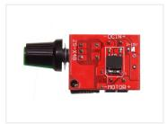
Extra compact PWM regulator for controlling the speed of a DC motor, with speed from 1% to 10%. Note that the motor will drop its performance as you lower the speed. This regulator will perform much better compared to just dropping the voltage.
