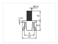
Cover strip with 10mm long  $\emptyset$  0.2mm brushes, that fit 8mm tracks, such as series 30 and 40 tracks. The brushes can be used for tightening, clean, guide and fix.
