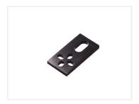
Aluminium plate for a microwitch, that then can be mounted on a V-slot so that it can function as an endstop. The microswitch is mounted in the 4 M3 holes. The placement of the holes makes it possible to turn the switch in various positions The oblong M5 hole is used for adjusting the endstop.
