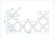
Very sturdy V-slot profile, typically called C-beam, primarily intended for larger machines requiring high stiffness, eg. CNC mills.
