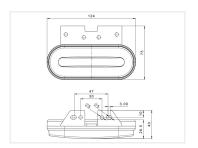
Nice marker lamp with LEDs in the middle and built-in reflex. The lamp is available in yellow, red and white and can be connected to both 12V and 24V. The powerful LEDs provide a clear marking on distance, and the reflector glass makes the car, truck or trailer visable - even when it's turned off.
