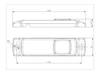
Nice and slim marker lamp with LEDs in the side and built-in reflex. The lamp is available in yellow, red and white and can be connected to both 12V and 24V. The powerful LEDs provide a clear marking on distance, and the reflector glass makes the car, truck or trailer visable - even when it's turned off.
