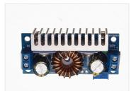
Compact step up DC boost converter with max 8A input current. The voltage can be boosted up to 42V, adjusted with the small potentiometer. Max current on the input is 8A, and 5A on the output.
