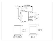
Contact with two contact sets / two poles, that can be used for many purposes, for example to swap polarity on motors.
