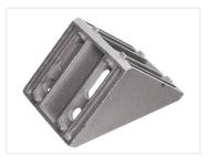
Large angle-bracket in cast aluminium for 6060 profiles in series 30, with two by two M8 mounting holes. The thickness of the bracket is 5mm.
