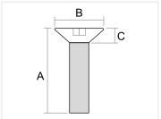
Bolt with countersunk head and for unbrako keys. For mounting in countersunk holes in brackets, hinges and similar.
