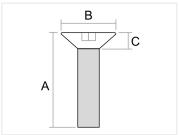
Bolt with countersunk unbracko head, for mounting in countersunk holes. Used in brackets, hinges and similar.
