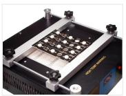
Preheater that is used for soldering or repairing circuit boards. It preheats the board so that components can be soldered or replaced easier. Typically you heat the board to +100 degree, where after you use a SMD hot air soldering station, or a soldering iron, to raise the temperature on the individual components, that need to be soldered or replaced.
