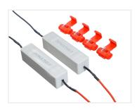
When switching the daytime running light buld with diode bulbs, the power consumption will be lower than usual and thare can be therefore experienced error messages on some newer cars with Can-Bus or bulb-control. You will therefore need to apply these "cheat resistors", which raise the consumption, so that it matches a regular bulb. The resistors will be connected to the + and - approach from the car.
