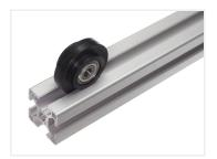
Wheel in hard plastic with a raised edge, that fits in to serie 30 and 40 tracks (8mm tracks). The wheel is used for guiding movable parts in the track of the aluminium profile. This could be a sliding door or similar. The wheel is made of durable nylon. The ball bearing ensures a smooth gliding motion, without wear.
