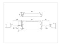
Box that is fixed or mounted temporary on your trailer with LED lamps. Built in resistors remove the most CANBUS errors on your car.
