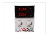
Powerful digitally adjustable laboratory power supply, 1 channel with max 30V and 5A. The voltage and current is easy to adjust with the two wheels, where a push on the wheel changes between which number is changed. The resolution of the voltage is 10mV, and the current is 1mA. The chosen setup is saved on restart.
