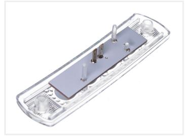
LED emitters 24V that replace the original circuits in the top lights on the new MAN trucks. The original emitters are taken apart by removing two metal clips, where after the board is taken out and the new put in.
