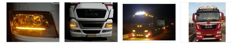
Complete kit for replaing the original white light in the DRL with yellow / amber light. The set consists of 2 boards, one for each side, and heat conductive paste to be used when mounting the boards on the original heat sinks.
