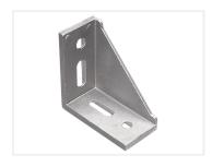
Extra large angle bracket, that gives extra stiffness and strength in the connection, compared to standard. There is space for 4 pcs M6 bolts in the bracket. You should use 14 or 16mm bolts together with a washer.
