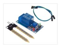
Sensor with controller that activates a relay, when the moisture falls under a defined value. The controller is easily adjusted with the small potentiometer.
