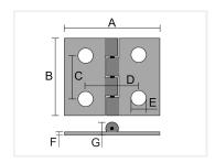
Hinges for series 30 in nylon and aluminium. Can be used for lids, movable parts and similar.
