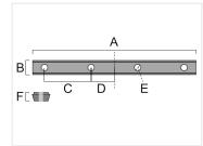
Strong solid alu-bar that fits in to 8mm series 30 slots. The bar is tightened between two profiles to join them. There are 4 pinol-screws that are used to fasten the bar.
