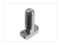
Hammer-bolt that fits in to the 8mm slots of series 30 profiles. The flat sides makes it possible to insert the bolts anywhere in the tracks. The bolt is turned 90 degrees in the slot where it is locked, where after it can be tightened.
