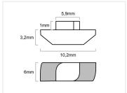
Nut that fits down in our series 20 profiles with 6mm slot. The nut turns and locks itself when tightened.
