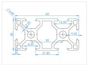
Strong alu-profile with basis dimensions 30x60mm, with two tracks on one side, and one on the other. The double width compared to the standard profile makes it extra useful for primary posts in constructions, or when you need two parallel tracks.
