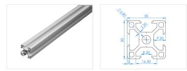
Standard profile in series 30, with basis dimensions 30x30mm and 8mm slot / track width. These profiles have a medium strength, and are a great choice for many types of constructions, such as CNC machines and automation tasks. The profile can also be used for CNC mills and automation tasks. The profile can also be used for shields, enclosures and similar.
