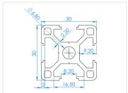
Standard profile in series 30, with basis dimensions 30x30mm and 8mm slot / track width. These profiles have a medium strength, and are a great choice for many types of constructions, such as CNC machines and automation tasks. The profile can also be used for CNC mills and automation tasks. The profile can also be used for shields, enclosures and similar.
