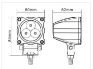
Powerful LED worklight in compact size, which still has a high output of 810 lumen. The black aluminium-housing protects LEDs, optics and electronics, and also works as a heat sink.
