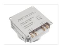
Smart and compact timer relay that is controlled by time and weekday, as well as workday/weekend and other patterns. The relay must be supplied with 12V, but the internal relay can switch 230V, up to 10A. The built-in backup battery, lets the watch tick without supply, with a life span of up to 3 years.
